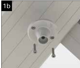
Tie bar at ridge Mark the position of where the tie bar meets the ridge, fix the ridge fixing cover using the self tapping screws provided.
