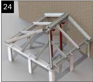
Ensure all gutter runs have been fitted and that all glazing bars are fully secured.
