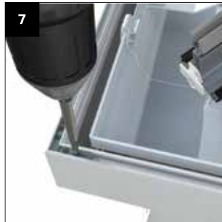
As shown in step 5 it may be advisable to temporarily support the Cornice whilst fixing. Secure corners using the cleats (CRN001) and fixings provided (CRN006).
