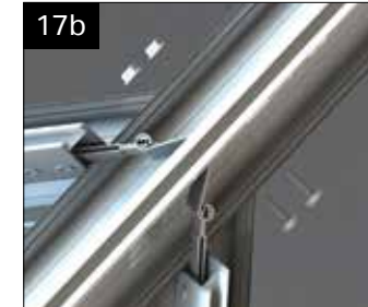
If two jack rafters are aligned either side of the hip, a M6 x 25mm bolt is required to fix both sets of brackets through either side.
