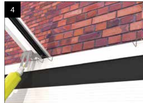
4 Fit brackets in marked positions on the bars as per standard installation and fit closure trims CHA---GR/5 according to layout plan.
