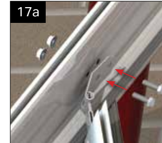
Align the bracket with the pre drilled holes on the hip bar, pass two M6 x 20mm through the holes and secure with flanged nuts.
