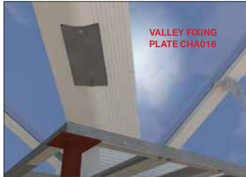
Mark out and cut the valley cladding and fix valley fixing plate by following steps 1 - 5.
