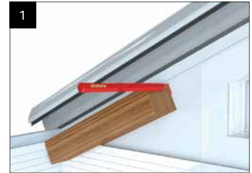
Using the location plan provided find the dimension for setting out the clip positions for the gable brackets. Measure up the bar from top edge of the fascia board and mark it.
