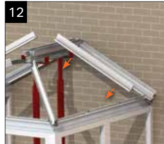
Continue to support the ridge and offer up the rafters that meet the ridge. Locate onto the double bolts at the ridge and bolts at the eaves.
