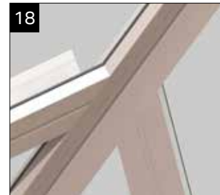
Once fixed, minor adjustment may be required to align the undercladding flush with the under side of the hip, this can be done by adjusting the bolts to suit. Repeat these steps until all jack rafters are fitted. Fully secure all rafters and hips.
