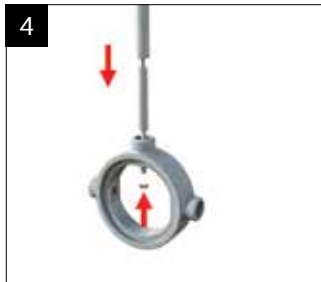
Insert the smaller diameter pieces of PVCu conduit inside. Offer into the boss ring and finger tighten the nyloc nut.
