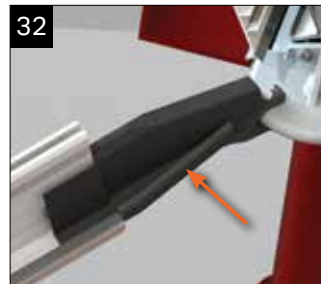
Fit the spider arm covers with the glazing seals inserted.
