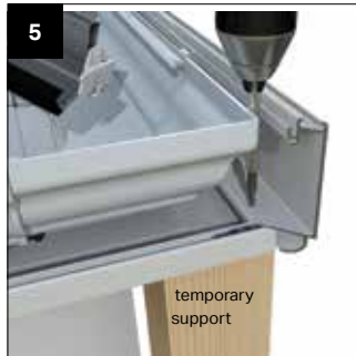
Offer up the middle Cornice section into position, (it may be advisable to temporarily support the lower Cornice section whilst fixing) secure using fixings provided (CRN007). (Long reach driver required).
