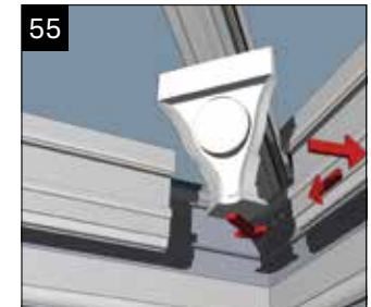
55 Fit the corner covers by trapping them behind the fascia sections. Insert the circular infill to finish.
