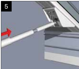
Offer up the horizontal pieces of PVCu conduit (large and small diameter).
