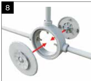
Offer up the two part rose cover, spin one half onto the threaded end of the other half.
