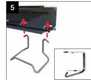
5 To retain the glazing to the valley wing, fit 2 wire clips (100mm from each end of the profile). The 'hooked ears' locate behind the lip detail as shown. Apply a continuous bead of sealant (MS Polymer to self cleaning glass). See Step 37 on page 16.
