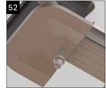
52 Offer up the internal radius end cap, use the threaded bar and the retaining boss to secure the internal cap in position. The threaded bar may require cutting to suit.
