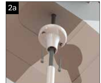
2a Offer up the internal radius end cap, retain this using the tie bar ridge fixing cover and two self tapping screws provided. Cut the PVCu conduit to suit.
