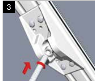
Measure, cut and attach the horizontal threaded bars (ensure sufficient engagement of the bar into the brackets) – it is essential that the tie bar boss is central. Take the boss ring, and loosely assemble the threaded bars to check they terminate inside the ring. Dis-assemble.
